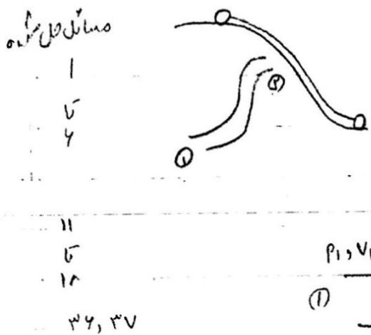
$$\frac{V_1^2}{\gamma g} + \frac{P_1}{\rho g} + h_1 = \frac{V_2^2}{\gamma g} + \frac{P_2}{\rho g} + h_2$$
