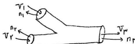
$$\times \frac{\partial}{\partial t} \int \rho d\mathcal{V} = \rho_1 V_1 A_1 + \rho_2 V_2 A_2 - \rho_3 V_3 A_3$$
