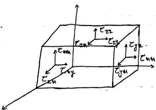
$$\left. \begin{array}{c} \sigma_{zz} \\ \sigma_{yy} \\ \sigma_{xz} \end{array} \right\} \leftarrow f_z \quad \left. \begin{array}{c} \sigma_{xy} \\ \sigma_{yz} \\ \sigma_{zx} \end{array} \right\} \leftarrow f_y$$
