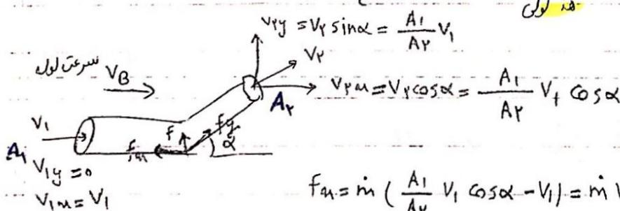
$$f_n = \dot{m} \left( \frac{A_1}{A_r} V_1 \cos \alpha - V_1 \right) = \dot{m} V_1 \left( \frac{A_1}{A_r} \cos \alpha - 1 \right)$$
